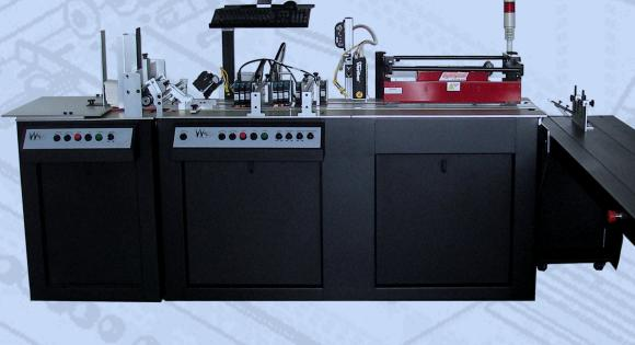
The series 655MB incorporates inkjet printing and drying systems on the same transport base. It was engineered for the high capacity use demanded by today's commercial environment. This versatile tranport system was designed for ease of use along with accuracy of product registration. The ergonomic operator panel allows for independent control of transport devices including dryer temperature control.
